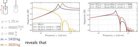
$-R(j\omega)$  vanishes at the resonance of  $\Delta_P$  at  $\omega = 5.31$ Therefore, this resonance isn't excited by r (incidentally). Yet the resonance of  $\Delta_P$  at  $\omega = 3.76$  isn't canceled.
