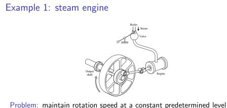
Problem: maintain rotation speed at a constant predetermined level Actuator: throttle valve can regulate the admission of steam into cylinders Obstacles: unpredictable changes (uncertainties), like
