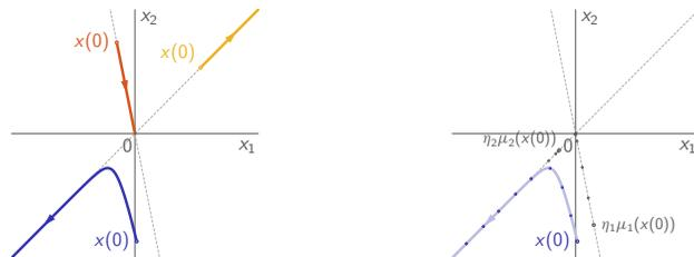
The initial conditions  $x(0) = \eta_1$  and  $x(0) = \eta_2$  generate the traverse of  $x(t)$  along the corresponding eigenvectors, while  $x(0) = -\eta_1 - 0.25\eta_2$  results in a superposition of two modes. Additional observations:
