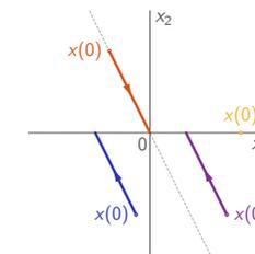
Starting on  $x(0) = \eta_2$  results in a point ( $x = x(0)$ ), other initial conditions generate the traverse along a line parallel to  $\eta_1$  and shifted by  $\mu_2(x(0))\eta_2$ , so all converge to  $\mu_2(x(0))\eta_2$ , like those from  $x(0) = \eta_1$ ,  $x(0) = -\eta_1 - 0.6\eta_2$ , and  $x(0) = -\eta_1 + 0.4\eta_2$ .
